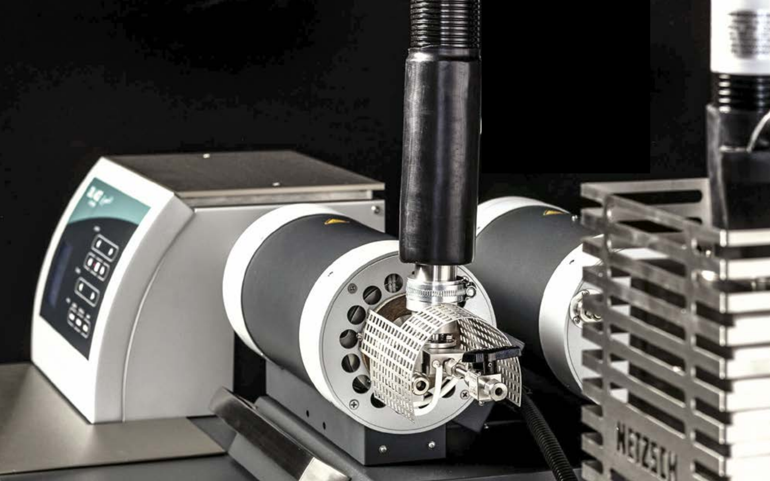
Silicon carbide furnace with transfer line connected for evolved gas analysis
